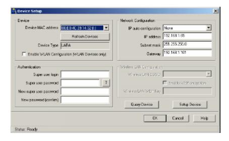
Figure 4-1. IP-KVM switch setup tool
